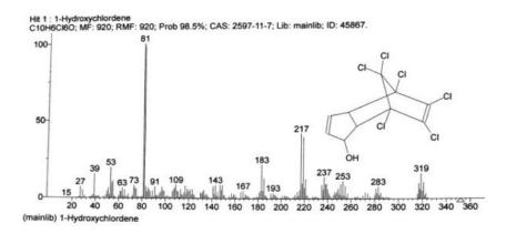
Figure 4: Chemical structure and mass spectra of metabolite 1-hydroxychlordene
